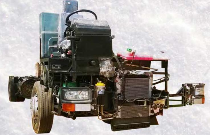
An optimized driveline allows you to cruise at higher speeds at lower engine revs for high efficiency & quiet running with significantly low noise levels. A Fully air suspended, rugged and torsionally rigid chassis designed for highly stable driving and excellent ride comfort. One of the safest and most effective braking systems consisting of Service brakes with ABS.
